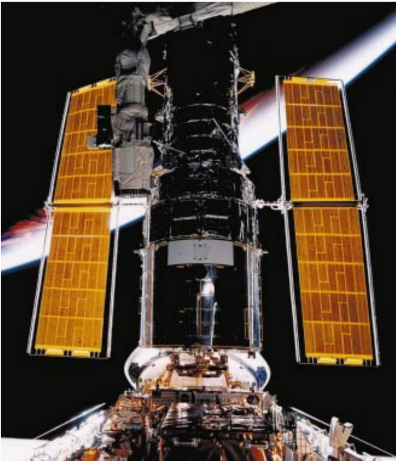
The Hubble Space Telescope in the cargo bay of the Space Shuttle during the last servicing mission
