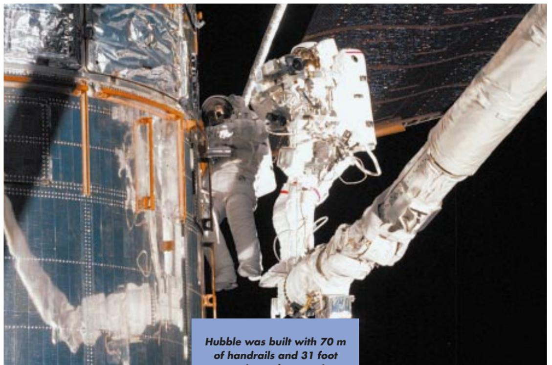
**Hubble was built with 70 m of handrails and 31 foot restraint sockets to give astronauts safe and convenient work sites as they hurtle around the Earth at 27,000 km an hour. On the ground that would be like travelling between two villages 7 km apart in a single second.**
