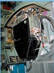
Wide Field Camera 3 (WFC3) Into Aft Shroud Radial Bay
