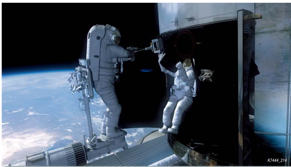
Fig. 2-13 Astronaut Mike Good, on the Shuttle RMS, moves a replacement RSU into place in the -V3 aft shroud doors. Astronaut Mike Massimino provides visual assistance to ensure precise alignment of the RSU on its mounting plate.
