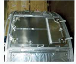
New Outer Blanket Layer (NOBL) insulation Onto Bays 5 and 8
