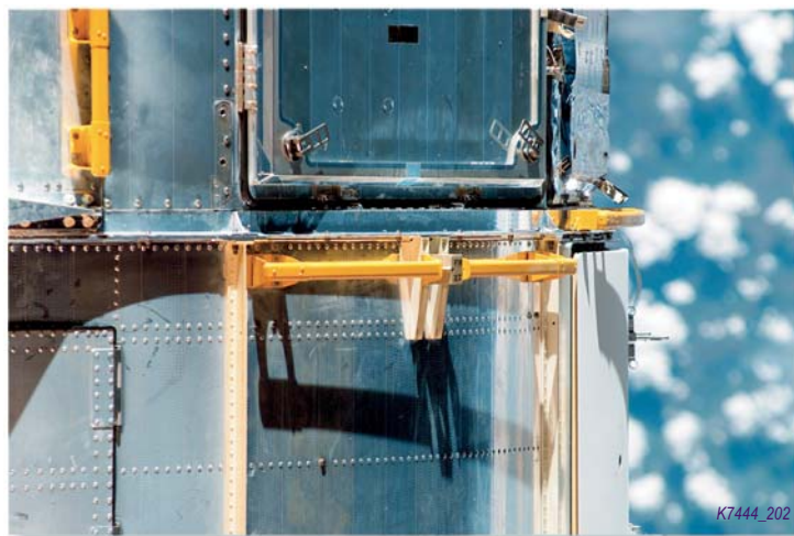
Fig. 2-2 The telescope has 225 feet of handrails to increase astronaut mobility and stability.
