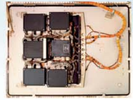
Science Instrument Command and Data Handling (SI C&DH) unit Into Bay 10
